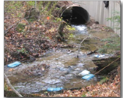
Figure 25. Six of the polymer blocks placed downstream
