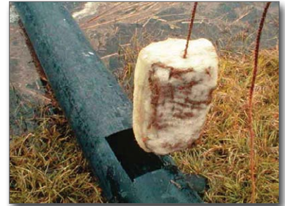
Figure 19. Polymer blocks inserted into pipes
