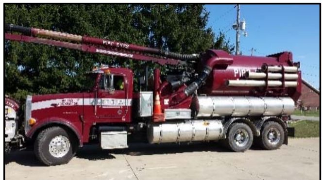
Combination Sewer Truck with 1,500 gallon water tank
