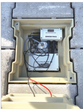
The INFIL-Tracker is a below pavement sensor.
