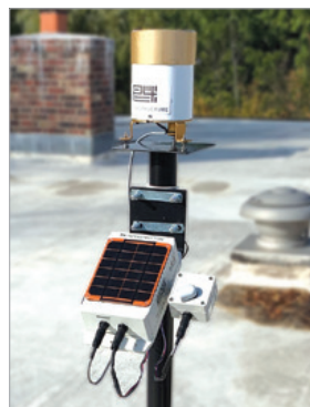
P4's INFIL-Tracker and Rain-mX transmit rainfall, stormwater captured, stormwater infiltrating, and when to clean the PaveDrain system.
