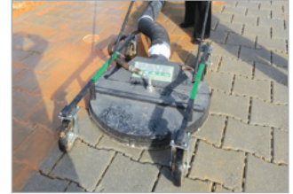
PaveDrain Vac Head shown above for small and hard to reach areas.
